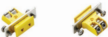
Type K ANSI illustrated (M29K-A). Recommended cutout: 6mm x 14mm
