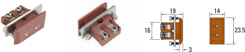
Type K illustrated (F34K). Recommended cutout: 8mm x 16.5mm
