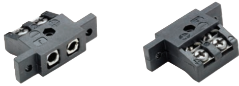
Type J IEC illustrated (R27J-I). Recommended cutout: 13mm x 26mm
