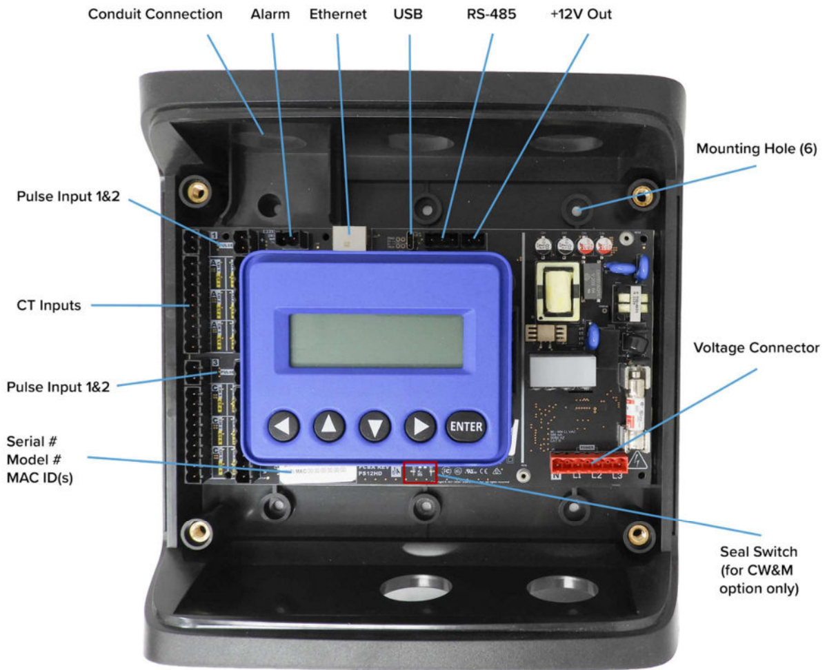
PS12HD (Enclosure with cover removed)
