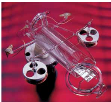
The 7250 Sys features a unique fused-quartz sensor. This rugged transducer offers unequalled precision and a stability of 0.0075% of reading per year.
