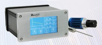
Chilled mirror hygrometry is a precise technique for determining the water vapor content is gases by directly measuring dew point or frost temperatures. Using this technique a metal mirror is cooled until it reaches a temperature at which a thin layer of condensation begins to form on it. The dew layer is detected optically, and the mirror is held at that temperature. The mirror temperature, measures with a PRT, is an accurate indicator of dew or frost point.
