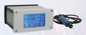
Chilled mirror dew point meter is a precise technique for determining the water vapor content is gases by directly measuring dew point or frost temperatures. Using this technique a metal mirror is cooled until it reaches a temperature at which a thin layer of condensation begins to form on it. The dew layer is detected optically, and the mirror is held at that temperature. The mirror temperature, measures with a PRT, is an accurate indicator of dew or frost point.
