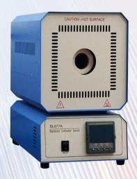
The BL677A is a benchtop blackbody calibration source utilizing a digital indicating temperature ambient 50 °C to 700 °C (122F to 1292F). A precision platinum RTD temperature sensor is embedded in the blackbody emitter, providing high accuracy and repeatability. The temperature controller uses the industry standard PID algorithms to control the emitter temperature to within 0.1°C of the set points.
