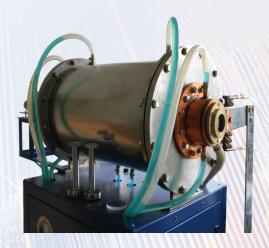
The BL681 is an ultra-high temperature blackbody calibration source system which utilizing a digital indicating temperature 400°C to 3000°C. A platinum rhodium wire sensor is embedded in the blackbody emitter, providing high accuracy and repeatability. The temperature to within 0.1°C of the set points. The black body emitter mechanism uses a resistive heating device that provides a long life, short stabilization times, and stable temperature control.
