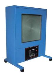
The BL690 series large area calibration source combine high temperature, unchangeable stability and perfect uniformity. The multi-segmentation temperature control provides a very precision and stable performance. Emitter source temperature control is carried out by a precision digital PID controller. User can pre-set 10 sets parameters to fast heat up the emitter. Eight different plat plate size is available, also custom design is possible.
