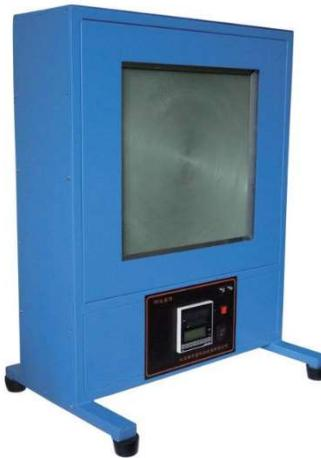
The BL690 series large area calibration source combine high temperature, unchangeable stability and perfect uniformity. The multi-segmentation temperature control provides a very precision and stable performance. Emitter source temperature control is carried out by a precision digital PID controller. User can pre-set 10 sets parameters to fast heat up the emitter. Eight different plat plate size is available, also custom design is possible.
