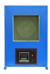
The BL690 series large area calibration source combines high temperature, unchangeable stability and perfect uniformity. The multi-segmentation temperature control provides a very precision and stable performance. Emitter source temperature control is carried out by a precision digital PID controller. Users can pre-set 10 set parameters to fast heat up the emitter. Eight different plate sizes are available, also custom design is possible.
