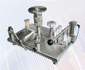
With high precision accuracy, the model BL502 pneumatic deadweight tester is ideal primary standard for defining the pressure scale in pneumatic range from 5kPa to 10MPa. The piston cylinder assembly is the heart of the dead weight tester and responsible for its high accuracy. Because of the extreme hardness of this material, the pressure distortion (expansion) coefficient is negligible. The low friction coefficient provides minutes of turning with just a little swing of the masses.
