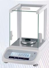
BL826 Precision Analytical Balances are highly accurate weighing instruments. Given the sensitivity of their high-performance weighing cells, these balances are equipped with a draft shield to maintain a stable weighing environment. With capacities up to 220 g and readability of 0.1 mg, these balances are ideal for applications such as sample and standard preparation, formulation, differential weighing, density determination, and pipette routine testing.
