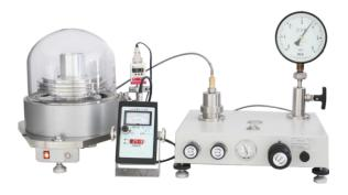
The gas operated BL503 absolute pressure piston gauges as primary standards for absolute pressure and gauge pressure, with emphasis on obtaining the effective area from the piston-cylinder dimensions and the mass in vacuum of the pressure balance floating element. It is designed to enable metrology and research institutes to realize and disseminate exceptional fundamental pressure measurements.
