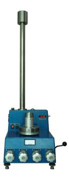
The BL504 liquid column pressure standard is a piston pressure vacuum gauge with a balanced liquid column. The working principle is based on that the pressure generated by the liquid column in the reservoir and pipeline is balanced with the initial pressure of the piston. Therefore, when measuring pressure, it can measure the pressure from zero. The BL504 is ideal for vacuum and low pressure calibration in primary metrology labs.
