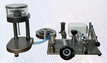
With high precision accuracy, the BL506 vacuum pressure deadweight tester have dual vacuum and pressure modes. Pressure and vacuum application can be operated by hand pump or external gas supply. To guarantee an excellent metrology-logic characteristics, all pistons and cylinders are made of extreme hardness tungsten carbide, the pressure distortion (expansion) coefficient is negligible. The low friction coefficient provides minutes of turning with just a little swing of the masses.
