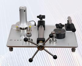
The model BL510 portable deadweight tester provide a precise means for generating pressure with high accuracy that can be used as a primary calibration standard. The unit's built-in shuttle valve provides the means to control the rate of pressure increase, while precision adjustment is accomplished with an integral micro vernier displacement valve. An ideal product that offers a rugged field ready primary standard, certified to yield consistent accurate results.
