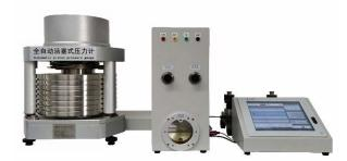
The model BL533 series automatic hydraulic piston gauge performs great pressure accuracy and an excellent long term stabilization as a primary standard. It is perfect solution in accredited pressure metrology institute and industrial pressure calibration laboratory.
