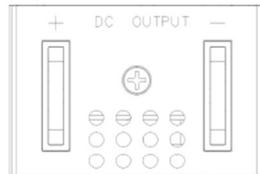
Output terminals for 6V to 60V models.
